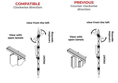
The above drawing should be interpreted as a front projection of the system.
